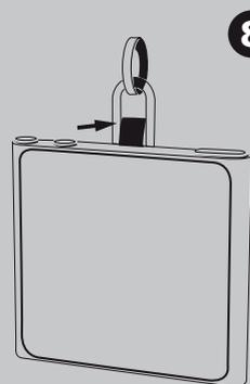
When removing the digems kit, push the tip lightly away from the ipod and the kit will slide away easily. As soon as the underneath of the body is visible the iPod clip can be pressed and the kit removed sideways.
